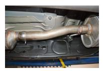
2. To remove stock exhaust, un clamp it at the connection behind the Y-pipe. Make sure to leave all rubber grommets in the factory location. **You will re-use stock clamp.** For easier removal of exhaust, cut behind the muffler. Use WD-40 to remove hangers from grommets.
