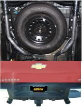
8. Install exit pipes #E onto tailpipes. Cut to your preferred length then use clamps to secure exit pipes to tailpipes. Install stainless steel tips. Clamp down.
