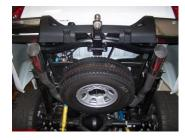
8. Install exit pipes #E. Use clamps #H to secure tailpipes. Do not tighten.
