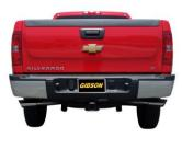
9. Install stainless steel tip. Clamp down. When you have everything in place, firmly tighten all bolts and clamps down securely. Use stainless steel cleaner and a Scotch Brite pad weekly to prevent tip from discoloration. Inspect all fasteners after 25-50 miles of operation and re-tighten as necessary.
