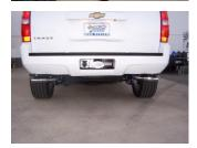
**8.** Install the exit pipes #E and #F. Use clamp #H to secure exit pipes to tailpipes. DO NOT TIGHTEN.
