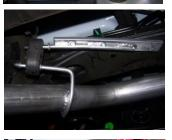
**9.** Install the exit pipes #E. Use clamp #H to secure exit pipes to tailpipes. DO NOT TIGHTEN.
