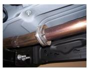
2. To remove stock exhaust, unbolt it at the flange behind the Y-pipe. Make sure to leave all rubber grommets in the factory location. You will reuse stock nuts and bolts. For easier removal of exhaust, cut behind the muffler. Use WD-40 to remove hangers from grommets.
