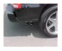
INSTALL YOUR BLACK CERAMIC COATED TIPS. PROCEED TO THE NEXT SHEET ON HOW TO INSTALL YOUR DEEGAN 38 BADGES. AFTER YOU HAVE CHECKED FOR CLEARANCES GO BACK AND TIGHTEN ALL NUTS, BOLTS AND CLAMPS...
