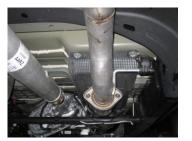
3. Install headpipe #A onto your existing stock 2-bolt flange. Use your factory nuts. Insert hanger into rubber grommet. Do not tighten. **On short beds cut 12.5" ofl headpipe**
