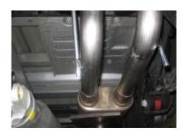
4. Install muffler #B onto headpipe #A 1.5-2" with louvers facing towards the converter. Use a jack stand to support the muffler. Use clamp #G to secure together. Do not tighten.
