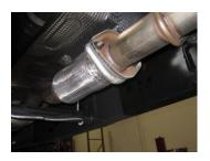
2. To remove your stock exhaust, unbolt the 2-bolt flange located in front of the muffler. Then cut off your tailpipe. Leave all rubber grommets in place.
