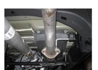
3. Install headpipe #A onto your existing stock 2-bolt flange. Use your factory nuts. Insert hanger into rubber grommet. Do not tighten.
