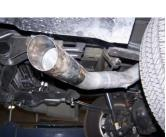
6. Slide passenger side tailpipe #C into muffler 1.5-2". Use clamp #H to secure. Do not tighten. Insert welded hangers into rubber grommets.
