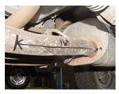
2. TO REMOVE STOCK EXHAUST, CUT 16" FROM THE FRONT OF THE MUFFLER FORWARD TOWARDS THE FRONT OF THE VEHICLE. LEAVE ALL RUBBER GROMMETS ON THE HANGER. USE WD-40 TO AID IN THE REMOVAL OF EXHAUST AND HANGERS.
