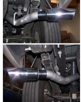
9. NEXT, INSTALL EXIT PIPES #F ONTO TAILPIPES USE CLAMP # J TO SECURE EXIT PIPES TO TAILPIPES.
