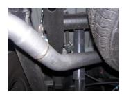
8. INSTALL DRIVER SIDE OVER AXLE TAILPIPE #D INTO THE MUFFLER. 11/2" TO 2" ROTATE PIPE UNTIL IT HITS THE 10"HANGER USE CLAMP # K TO HOLD UP THE PIPE, ATTACH TAILPIPE TO MUFFLER USING CLAMP # H. DO NOT TIGHTEN.
