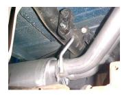
5. NEXT, INSTALL REAR MUFFLER HANGER #H ONTO DRIVER SIDE OUTLET OF THE MUFFLER. INSERT HANGER INTO RUBBER GROMMET DO NOT TIGHTEN.
