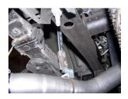
6. MEASURE 18" FROM THE REAR OF THE FRAME TOWARDS THE FRONT OF THE VEHICLE. USE THIS SLOT FOR THE 10" HANGER #K, INSTALL USING THE 1ST HOLE USE HARDWARE KIT #L.
