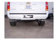
Inspect all fasteners after 25-50 miles of operation and re-tighten as necessary.
