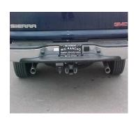
Install driverside overaxle tailpipe #E into muffler 1 ½" to 2". Use clamp #I to secure pipe to muffler. Do not tighten. Next, insert welded hanger into rubber grommet. Rotate pipe until it connects with rear hanger. Attach clamp #I to tail pipe.
