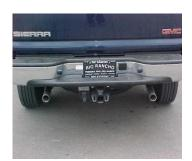
Install passenger side overaxle tailpipe #D into muffler 1  $\frac{1}{2}$ " to 2". Secure with clamp #H. Do not tighten.
