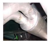
Lay out the exhaust on the floor so it looks like the drawing and compare parts with manual. **To remove the stock exhaust cut 13" just in front of the muffler.** Leave all rubber grommets in place. Use WD-40 to aid in removal of exhaust and hangers. Use hacksaw to
