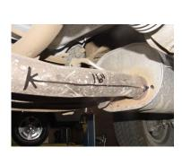
SLIDE PASSENGER SIDE HEADPIPE #A ONTO STOCK HEADPIPE. INSERT WELDED HANGER INTO RUBBER GROMMET. NEXT INSTALL DRIVERS SIDE HEADPIPE # B, AND USE CLAMP #I TO SECURE BOTH HEADPIPES. DO NOT TIGHTEN.
