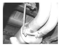
Install hanger #I onto the rear outlet of the muffler on the driver side. Insert the vertical rod through the rubber grommet from the driver side towards the passenger side. Do not tighten.
