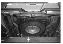
Install exit pipes # E onto the over axle pipes and attach with clamp #G. You may need to cut the exit pipes to your preference. Rotate all pipes until you have a minimum of a 1" clearance on all pipes. Use zip ties to reroute vent lines and brake lines. Tighten all clamps, flanges, bolts firmly. Install Stainless steel tips.
