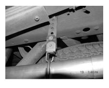
REMOVE STOCK REAR HANGER FROM FRAME ON PASSENGER SIDE. INSTALL 10" METAL HANGER #I. USE THE FIFTH HOLE FROM THE BOTTOM. INSTALL IT IN THE TOP FACTORY HOLE WHERE THE STOCK HANGER WAS IN. IT IS LOCATED APPROX. 20" FROM REAR OF FRAME 3/8" HOLE.REPEAT FOR THE DRIVERSIDE.
