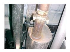
YOU MAY NEED TO HEAT IT UP FOR EASIER REMOVAL. LEAVE ALL RUBBER GROMMETS IN PLACE. USE WD-40 TO AID IN REMOVAL OF EXHAUST AND HANGERS.
