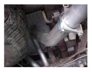
Install metal hangers # I Into holes located approximately 22" from the rear of the frame. Metal hangers are mounted on the outside of the frame. Use bolt kit #K. The bolt and the washer will go into the 3<sup>rd</sup> hole from the top of the hanger.
