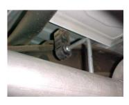
onto you're existing stock flange use your factory hardware. Use a jack stand to support the converter. Insert welded hanger into rubber grommet. Do not tighten.
