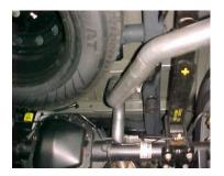
INSTALL OVERAXLE TAILPIPE #C INTO MUFFLER 1 ½" TO 2". INSERT HANGERS INTO
