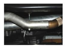
2. INSTALL HEADPIPE #A ONTO THE FACTORY EXTENSION PIPE. INSERT WELDED HANGER INTO RUBBER GROMMET. USE CLAMP #E TO ATTACH IT TO THE FACTORY EXTENSION PIPE. DO NOT TIGHTEN
