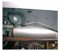
INSTALL MUFFLER # B ONTO HEADPIPE  $1\frac{1}{2}$ " TO 2". USE CLAMP # E TO SECURE MUFFLER TO HEADPIPE. DO NOT TIGHTEN. USE A JACK STAND TO HOLD UP THE MUFFLER. MUFFLER INLET IS LOOKING INTO THE LOUVERS. OUTLET SHOULD BE AT T HE 10 O'CLOCK POSITION.
