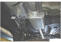
4. Install muffler #B onto headpipes #A 1.5-2" with the louvers facing towards the converter. Use a jack stand to support the muffler. Use clamp #G to secure the muffler to the headpipes. Do not tighten. Muffler inlet is looking into the louvers.
