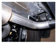
5. Install extension pipe #C onto muffler outlet. Use clamp #H to secure the pipe to the muffler.
