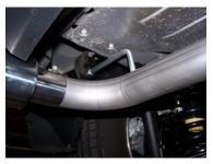
7. Install muffler assembly #E onto extension pipe. Insert hangers into rubber grommets. Use clamp #H to secure pipes together. Do not tighten.
