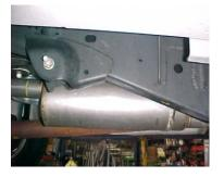
INSTALL MUFFLER # B ONTO HEADPIPE 1  $\frac{1}{2}$ " TO 2". USE CLAMP # E TO SECURE MUFFLER TO HEADPIPE. DO NOT TIGHTEN. USE A JACK STAND TO HOLD UP THE MUFFLER. MUFFLER INLET IS LOOKING INTO THE LOUVERS. OUTLET SHOULD BE AT T HE 10 O'CLOCK POSITION.
