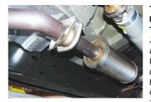
TO REMOVE YOUR STOCK EXHAUST, REMOVE IT FROM THE 2 BOLT FLANGE LOCATED JUST IN FRONT OF THE MUFFLER AND REMOVE HANGERS FROM RUBBER GROMMETS BY PULLING EXHAUST TOWARDS THE REAR OF THE VEHICLE, USE WD-40 TO AID IN REMOVAL, LEAVE GROMMETS IN PLACE.
