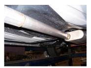
5. Install extension pipe #C onto muffler outlet. Use clamp #H to secure the pipe to the muffler. Insert welded hanger into rubber grommet.
