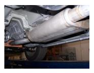
4. Install muffler #B onto headpipe #A 1.5-2" with the louvers facing towards the converter. Use a jack stand to support the muffler. Use clamp #H to secure the muffler to the headpipe. Do not tighten. Muffler inlet is looking into the louvers.
