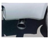
**8.** Install stainless steel tip #E. Clamp down. When you have everything in place, firmly tighten all bolts and clamps down securely. Use stainless steel cleaner and a Scotch Brite pad weekly to prevent tip from discoloration.
