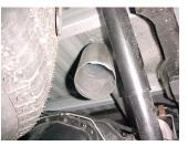
**5.** Install the over axle tailpipe #C into the muffler  $1\frac{1}{2}-2^{"}$  and secure with clamp #G. DO NOT TIGHTEN.
