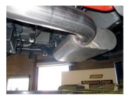
4. Once you have entire system hanging loose re install the factory fram support bracket. Instal the forward bolt loosly and used the supplied spacers and bolts for the rear 6 bolts. Tighten down all the bolts.
