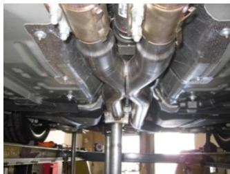
2. Install your Gibson x-pipe using the stock clamps. Be sure to keep loose until the entire system is in place.
