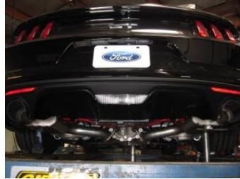
5. Check for clearance on all pipes and tip location. Place rubber objects or wood objects in areas that have little clearance. This will help hold the exhaust in place when you begin to tighten everything down. Once you have everything in place, firmly tighten all bolts and clamps down securely. Remove objects holding parts in place and double check all clearances.
