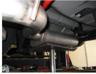
3. Now install the passenger side muffler assembly #B by sliding the metal hangers into the rubber grommets. Then do the same for the driver side muffler assembly #A. Use clamp #D to secure together. Keep loose.
