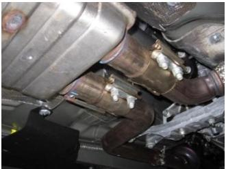
2. To remove your stock exhaust, unbolt it from the clamps located just after the manifolds then remove the whole exhaust system
