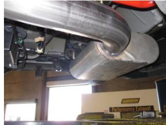
4. Once you have entire system hanging loose re install the factory fram support bracket. Instal the forward bolt loosely and used the supplied spacers and bolts for the rear 6 bolts. Tighten down all the bolts.
