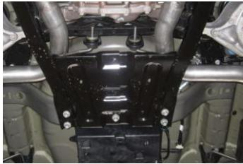
1. Prior to removing your factory exhaust you we will need to remove the factory directly behind the rear diff and runs outward towards each vehicle door. There is a combined 8 bolts that need to be removed.
