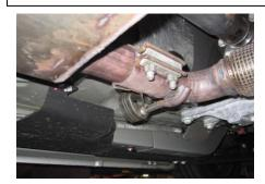
5. Now do the same procedure for the driver side. Use clamp # D to secure to the muffler. When you have everything in Place, firmly tighten all bolts And clamps down securely. Be sure you keep an eye on the tip position as it can move during the tightening process,
