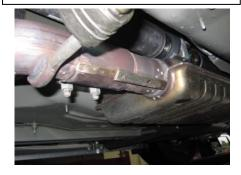
4. Now install the passenger side tailpipe assembly #B by sliding the metal hangers into the rubber grommets. Then do the same for the driver side muffler assembly #A. Use clamp #D to secure together
