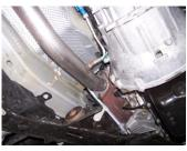
GIBSON EXHAUST systems are designed on a factory stock vehicle. Any aftermarket products installed could increase the sound levels of the exhaust. Make sure there is a 1" clearance from ALL rubber brake lines, shock boots, lines, tires, etc. to prevent heat related damage or fire.
