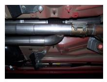
7. After kit is installed, adjust your kit so it does not hit or rub on anything. Check that your exhaust tips are not touching your bumper. After checking everything, now tighten all clamps starting from the front and working your way to the rear. Use stainless steel cleaner and a Scotch Brite pad weekly to prevent tip from discoloration. Inspect all fasteners after 25-50 miles of operation and re-tighten as necessary.
