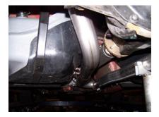
6. Install h-pipe adapter onto tailpipes. Use your factory clamp to attach it to your stock pipe. Do not tighten. Use clamps #D to attach your adapter to your tail pipe. Do not tighten.
