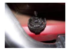
4. Now you are going to install the system in reverse order. First, install your new Gibson mufflers. There are specific left and right assemblies. Install rear muffler hangers using bolts from rubber grommet hanger. They are self-tapping bolts.
