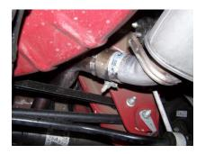
3. Next, remove the factory hanger from the rear and re-install on the driver side. Use your factory bolts, they are self-tapping. So you should have no problem re-installing the hanger. (see picture) Remove rubber grommet hanger. Do not discard bolts, you will re-use. (see picture)
