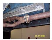
LAY OUT THE EXHAUST ON THE FLOOR SO IT LOOKS LIKE THE DRAWING AND COMPARE PARTS WITH MANUAL. TO REMOVE THE STOCK EXHAUST REMOVE IT FROM THE 2-BOLT FLANGE LOCATED IN THE FRONT OF THE MUFFLER. LEAVE ALL RUBBER GROMMETS IN PLACE. USE WD-40 TO AID IN REMOVAL OF EXHAUST AND
