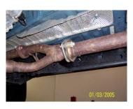
LAY OUT THE EXHAUST ON THE FLOOR SO IT LOOKS LIKE THE DRAWING AND COMPARE PARTS WITH MANUAL. TO REMOVE THE STOCK EXHAUST REMOVE IT FROM THE 2-BOLT FLANGE LOCATED IN THE FRONT OF THE MUFFLER. LEAVE ALL RUBBER GROMMETS IN PLACE. USE WD-40 TO AID IN REMOVAL OF EXHAUST AND HANGERS.
