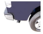
8. Install stainless steel tip. Clamp down. When you have everything in place, firmly tighten all bolts and clamps down securely. Use stainless steel cleaner and a Scotch Brite pad weekly to prevent tip from discoloration. Inspect all fasteners after 25-50 miles of operation and re-tighten as necessary. You may need to cut your stock tail pipe back to get your tip to fit correctly.
