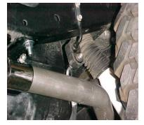
INSTALL THE OVERAXLE TAILPIPE #B INTO THE MUFFLER 1 ½" TO 2". SECURE TO THE MUFFLER USING CLAMP #D. DO NOT TIGHTEN. INSERT WELDED HANGERS INTO RUBBER GROMMETS. NOTE, SHORT END OF OVER AXLE PIPE INSERTS INTO MUFFLER.
