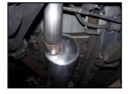
**3.** Install the Gibson muffler in the same position as the stock muffler and clamp to stock pipe with clamp #D. Muffler may angle down at back. Inlet of muffler is looking into the louvers. DO NOT TIGHTEN.
