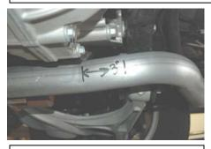
2. To remove the factory exhaust measure from the rear bend 3" forward. Please reference picture for location. Mark and cut with a hack saw or cut off wheel. Leave the factory rubber grommets in place they will be reused.
