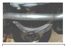
2. To remove the driver side exhaust measure 8" from the bend located under the rear end forward. Mark and cut with a hack saw or cut off wheel. Leave the factory rubber grommets in place they will be re used.
