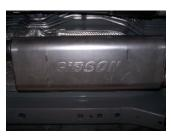
3. Install muffler #B onto headpipe #A 11/2-2" with the louvers facing towards the converter. Use a jack stand to support the muffler. Use clamp #F to secure the muffler to the headpipe. DO NOT TIGHTEN.
