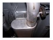
**4.** Install extension pipe #C into the muffler 11/2-2". Insert welded hanger into rubber grommet. Secure to muffler with clamp #F. DO NOT TIGHTEN.
