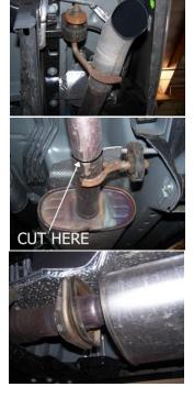
1. To remove the stock exhaust remove the nut on the rear hanger using a 21mm wrench, then cut the tailpipe just after the rear muffler hanger and remove. Unbolt the headpipe at the flange and remove. Leave all rubber grommets in place. Use WD-40 to aid in removal of hangers from rubber grommets.
