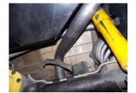
6. Install the over axle tailpipe #C into the muffler 1.5-2". Use clamp #E to secure tailpipe to muffler. Insert welded hangers into rubber grommets.
