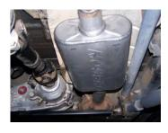
4. Install muffler #B onto headpipe #A 1.5-2" with the louvers facing towards the converter. Use a jack stand to support the muffler. Use clamp #D to secure the muffler to the headpipe. Do not tighten. Muffler inlet is looking into the louvers.
