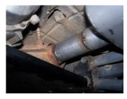
3. Install headpipe #A onto your existing stock pipe. This pipe will have to be welded to the converter. See picture.
