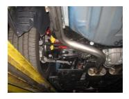
4. Install driver side tailpipe/ dual tip assembly #B. Insert all welded hangers into rubber grommets. Secure tailpipes with clamp #D. Do not tighten.
