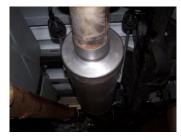
4. Install head pipe #A onto factory pipe. Use clamp #D to secure pipes together. Insert welded hangers into rubber grommets. Do not tighten.
