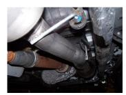
5. Install muffler #B onto head pipe #A 1½"-2" with the louvers facing towards the converter. Use a jack stand to support the muffler. Use clamp #D to secure the muffler to the head pipe. Do not tighten. Muffler inlet is looking into the louvers.
