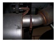
2. Remove your stock tail pipe from stock muffler by removing the clamp located on the outlet of muffler. Do not cut or damage your factory tail pipe you will re-use it. Leave all rubber grommets on the factory hangers on the vehicle.
