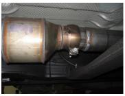
4. Install head pipe #A onto factory pipe. Use factory clamp to secure pipes together. Insert welded hanger into rubber grommet. Do not tighten.
