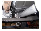
**3.** Install head pipe #A onto your existing stock flange and attach using the stock hardware. DO NOT TIGHTEN. Insert welded hanger into rubber grommet.
