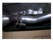
2. To remove the stock exhaust, unbolt the 2 bolt flange located in front of the new muffler. Disengage the welded hangers using WD-40 from the OEM rubber grommets. Do not damage or remove the rubber grommets as you will reuse them to mount your new system. Now, cut off tailpipe and remove exhaust.
