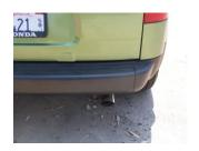
**11.** Install stainless steel tip. Clamp down. When you have everything in place, firmly tighten all bolts and clamps down securely. Use stainless steel cleaner and a Scotch Brite pad weekly to prevent tip from discoloration.
