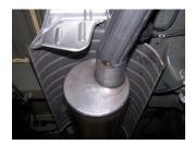
**4.** Install muffler #B onto headpipe  $1\frac{1}{2}$ "-2" with the louvers facing towards the converter. Use a jack stand to support the muffler. Use clamp #E to secure the muffler to the headpipe. Do not tighten. Muffler inlet is looking into the louvers. Outlet of muffler will be at approximately 2 oʻclock.
