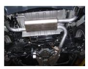
3. Install muffler assembly onto factory pipe. Insert hangers into rubber grommets. Use clamp #B to secure pipes together. Do not tighten.
