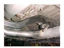
LAY OUT THE GIBSON EXHAUST ON THE FLOOR AND COMPARE PART #'S TO THE DRAWING. TO REMOVE YOUR FACTORY EXHAUST UN-BOLT YOUR TAILPIPE AT THE 2-BOLT FLANGE LOCATED BEHIND YOUR STOCK MUFFLER USE WD-40 TO AID YOU IN REMOVAL OF HANGERS FROM RUBBER GROMMETS. DO NOT DAMAGE THE GROMMETS, THEY WILL BE USED TO INSTALL THE NEW KIT NEXT, UN-BOLT YOUR EXHAUST FROM THE 2-BOLT FLANGES LOCATED JUST BEHIND YOUR FACTORY CATALYTIC CONVERTERS, DO NOT DISGUARD YOUR FACTORY GASKETS AND HARDWARE YOU WILL **RE-USE IT.**
