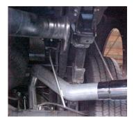
INSTALL OVERAXLE TAILPIPE # D INTO MUFFLER 1 ½"-2" INSERT WELDED HANGER INTO RUBBER GROMMET USE CLAMP # G TO SECURE PIPE TO MUFFLER.
