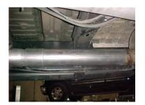
INSTALL EXTENSION PIPE #I ONTO HEADPIPE INSERT WELDED HANGER INTO RUBBER GROMMET USE CLAMP #G TO SECURE. DO NOT TIGHTEN.
