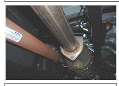
2. Be sure to not damage the gasket and bolts they will be re used for the exhaust install. (MAKE SURE TO REMOVE THE EXHAUST SENSOR LOCATED ON THE OVER AXLE PORTION OF YOUR FACTORY EXHAUST YOU WILL NEED A 15/16")
