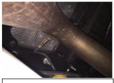
4. Install Over axle pipe Item # B onto the head pipe. Use clamp Item E to secure but do not tighten. Using the 15/16" wrench reinstall the exhaust sensor on the over axle pipe.
