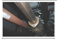
2. Be sure to not damage the gasket and bolts they will be re used for the exhaust install. (MAKE SURE TO REMOVE THE EXHAUST SENSOR LOCATED ON THE OVER AXLE PORTION OF YOUR FACTORY EXHAUST YOU WILL NEED A 15/16")
