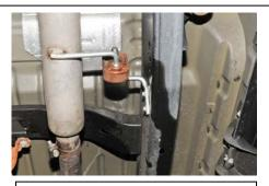
3. Install muffler assembly Item # A into the head pipe #F using clamp # E.Install hanger into rubber grommet and loosely tighten down the clamp. With the muffler assembly installed you may want to use a jack stand to support the muffler.
